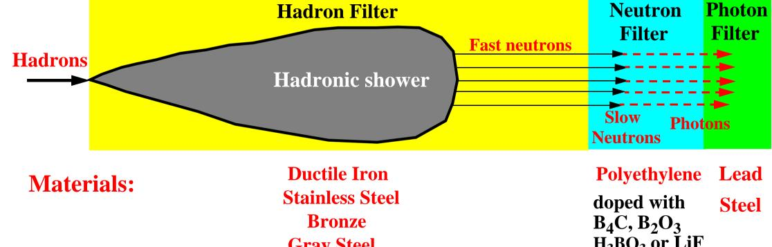
H<sub>3</sub>BO<sub>3</sub> or LiF **Gray Steel Thickness: 10-20 Interaction lengths** 5-8 cm **3** cm
